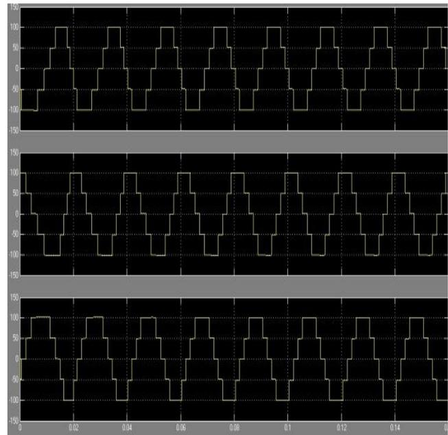
Fig.11. Phase to Phase Inverter voltages.
