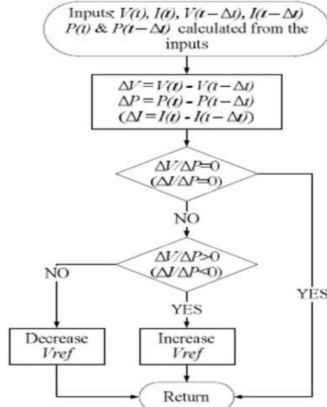
**Fig.5. Flow chart for the P&O method.**
