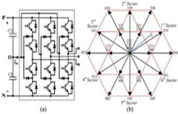
**Fig.3. Three level inverter circuit and its SPVWM diagram.**
