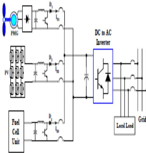
Fig.1. Configuration of Hybrid System.
