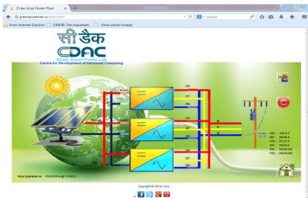
Fig. 6. Screen shot of on-line HMI.
